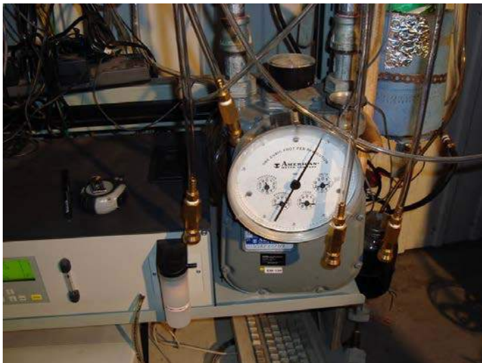
Picture 8: Reference dry gas meter
