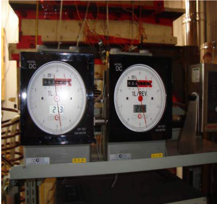
Picture 11: Dry gas meter
