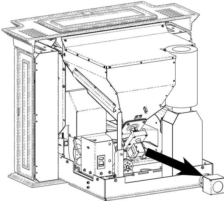
2. Connect the "Plate with pipe plug" with the inlet air pipe of the insert, then fix "Plate with pipe plug" on the sliding frame of the insert, fixing it with two screws as shown in the figure hereunder.
